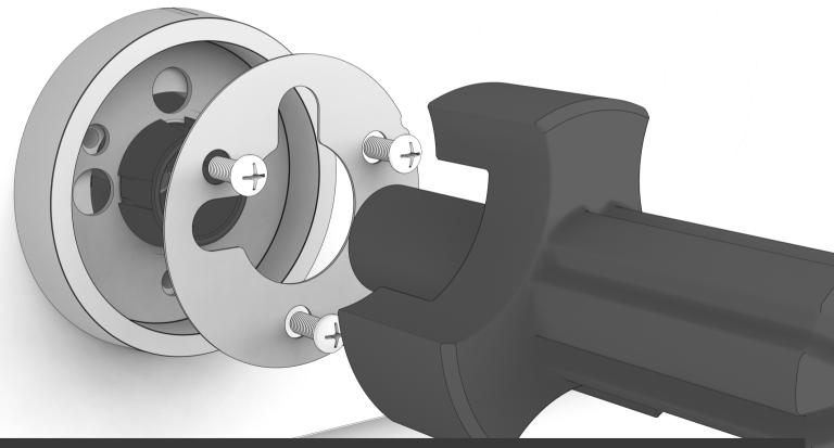
IF THE FLANGE IS PRESENT, REPOSITION IT IN THE CORRECT POSITION
