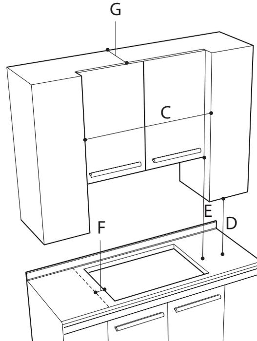
WALL COVERING CABINETS, AND COUNTERTOP MUST WITHSTAND HEAT UP TO 93° C (200° F)
