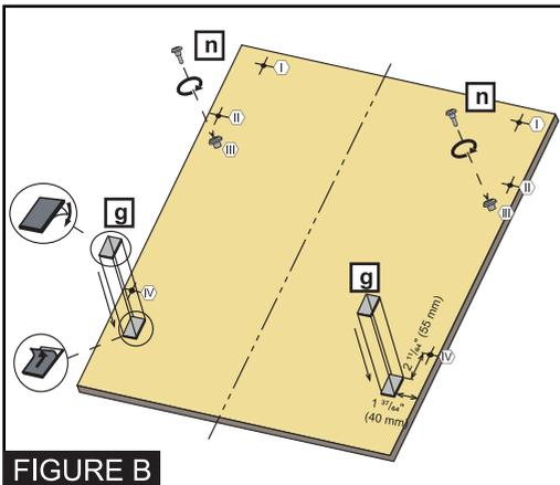
3- As shown in Figure B, Screws  $\varnothing$  5/32" x 27/32" ( $\varnothing$  4mm x 21,5mm) is installed in positions III.
