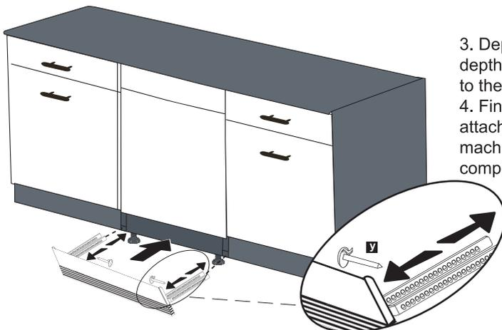
3. Depending on the desired depth, plinth locking(y) is attached to the toe kick bracket(o).
