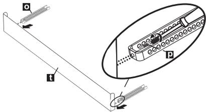
1. A. If the height is 33 7/8" to 35 7/8" (860mm-910mm) and use short supports; adjustable plinth metal with 80 mm length (v), toe kick brackets(o) are installed. Mounting is done using Screws  $\varnothing$  5/32" x 7/32" ( $\varnothing$  4mm x 6mm) with a Philips Screwdriver.
