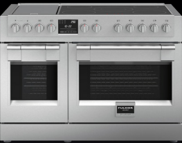
NEW INDUCTION RANGE 48" Knob Controlled 4 Single Induction cooking zones 1 Dual Max Power with Ø 11" zone 1 integrated trillaminate Griddle over a dedicated 2-zone bridge element Self-cleaning, Dual True Convection ovens Cool to the touch, soft closing door CODE ID F6PIR485GS1
