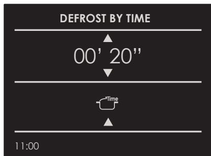
Once the function has been started, a countdown will be shown on the display. The time can be changed at any time using the arrows  $\Delta$  and  $\nabla$ .
