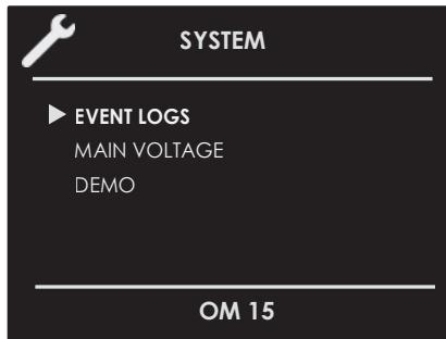
The purpose of this function is to set the DEMO mode, which makes the oven useless for cooking but automatically performs a demonstration of functions.
