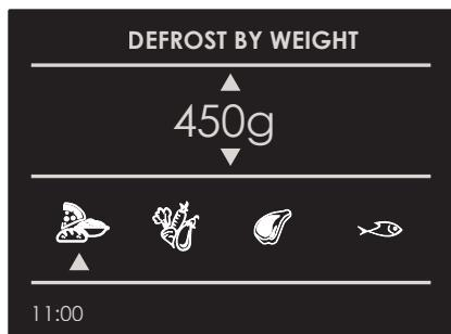
Select the type of meal using the arrows  $\triangleleft$  and  $\triangleright$ , then set the weight using the arrows  $\Delta$  and  $\nabla$ , finally start thawing using the key **OK**.
