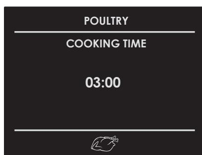
4. At this point, the recipe can be saved in the list of "PERSONAL" recipes by selecting "SAVE" and confirming by means of the **OK** key.
