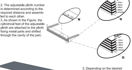
Depending on the desired depth, plinth locking(y) is attached to the toe kick bracket(o).
