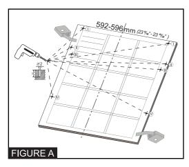
1. The mounting plan in the plastic bag is fixed to the inside of the Dishwasher door.
