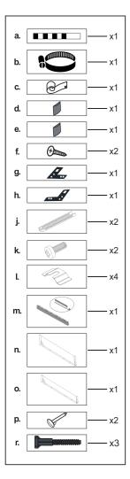
The parts required for positioning the dishwasher are in plastic bags. Check that all of the following parts are contained in plastic bags.
