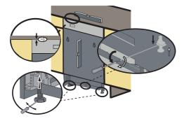
If the height of the enclosure is 33 7/8" to 35 7/8" (860mm-910mm) use short supports as shown in the figure.
