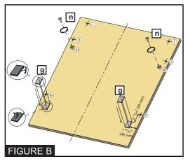
3- As shown in Figure B, Screws Ø 5/32" x 27/32" (Ø 4mm x 21,5mm) is installed in positions III.
