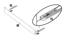
1. A. If the height is 33 7/8" to 35 7/8" (860mm-910mm) and use short supports; adjustable plinth metal with 80 mm length (v), toe kick brackets(o) are installed. Mounting is done using Screws Ø 5/32" x 7/32" (Ø 4mm x 6mm) with a Philips Screwdriver.
