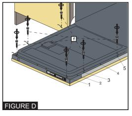
7- As shown in Figure D, Screws Ø 5/32" x 53/32" (Ø 4mm x 42,5mm) is installed in positions I,III and V.
