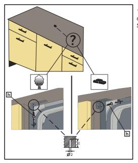
10- Mounting brackets previously fixed to the dishwasher are also fixed in the cabinetry with Screws Ø 5/32" x 19/32" (Ø 4mm x 15mm).
